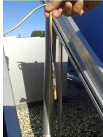
Figure 12: Broken temperature sensor of the collector, office building in Rohrbach, Austria
