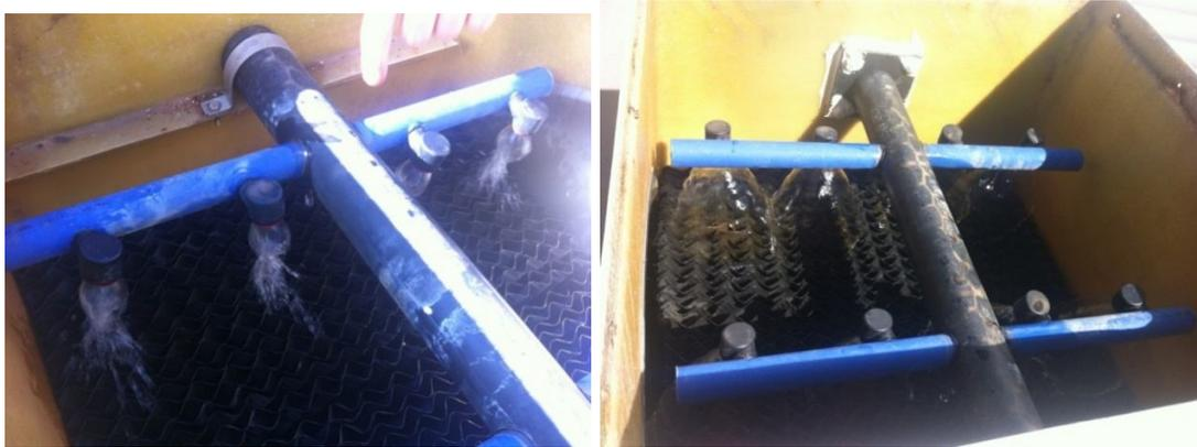
Figure 17: Water spraying at 1.5 m<sup>3</sup>/h (left) and 3 m<sup>3</sup>/h (right) (source: (Dalibard, 2014))
